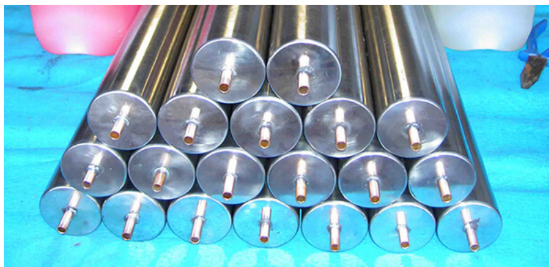
Fig. 9. Cylindrical encapsulation for PCM [17]
