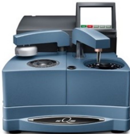
Fig. 2. DSC instrument (Make: TA Instruments, Model: Q1000) [11]
